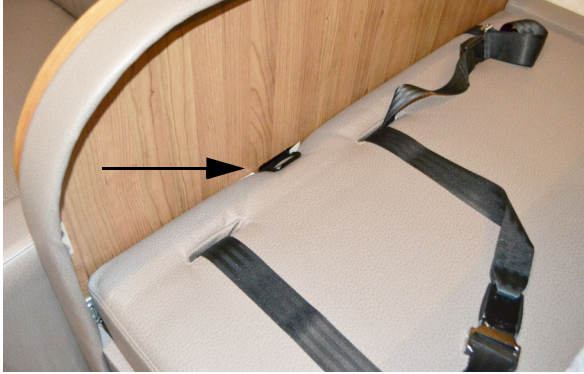
Tether Anchor Loop (Located behind the forward facing dinette seat back cushion)
