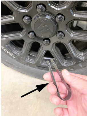
OEM lug bolt cover removal tool. -Typical View
